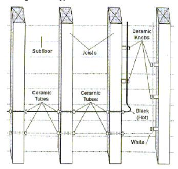
Diagram F1- Typical knob and tube installation
